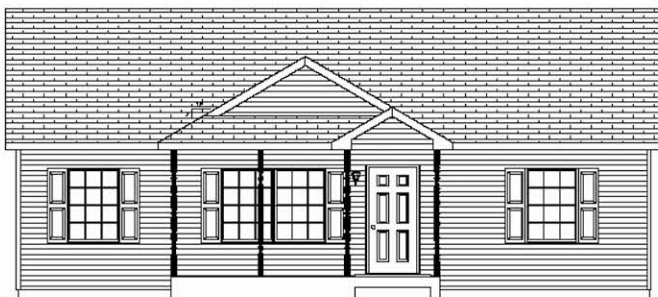
Decorative Dormer w/ 6' Porch Overhang w/ Hip Corner, Decorative Shingle Returns and False "A" Return
